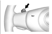
The Manual Paddle Shift system is activated from S (Sport Mode) by pushing the paddle, above the steering wheel spokes, to up-shift to the next gear, or pulling on the paddle, behind the steering wheel spokes, to down-shift to the next gear.
